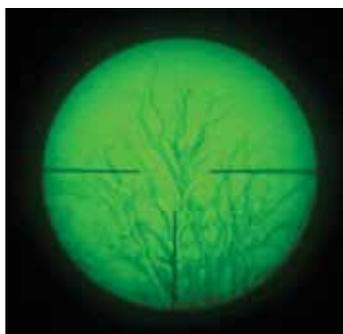
**A dead tree at 100m at 5x. The shading around the edges of the image is the result of imperfect camera alignment and isn't seen with the naked eye.**
