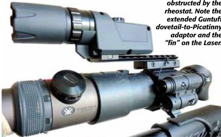
*Set up on the Vortex, the DSA isn't obstructed by the rheostat. Note the extended Guntuff dovetail-to-Picatinny adaptor and the "fin" on the Laser.*
