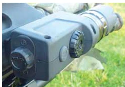
*The battery compartment cover is clearly marked for polarity, whilst a small rubber ON/OFF button and a larger black dial control the power and intensity of the laser, and locking ring lets you zero the beam.*
