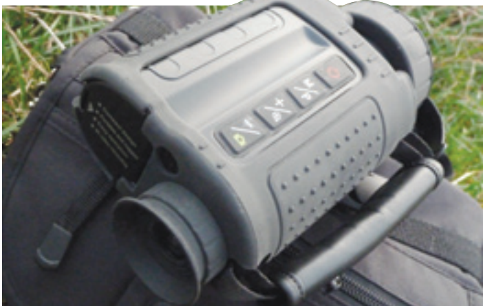
A rubber jacket provides a secure and comfortable grip and protects the alloy body of the camera from knocks and scratches. Note the eye-sensor opening between the ocular lens and the battery cover. Also note the four buttons that control the camera's functions. P is for "polarity" (bHOT/wHOT)
