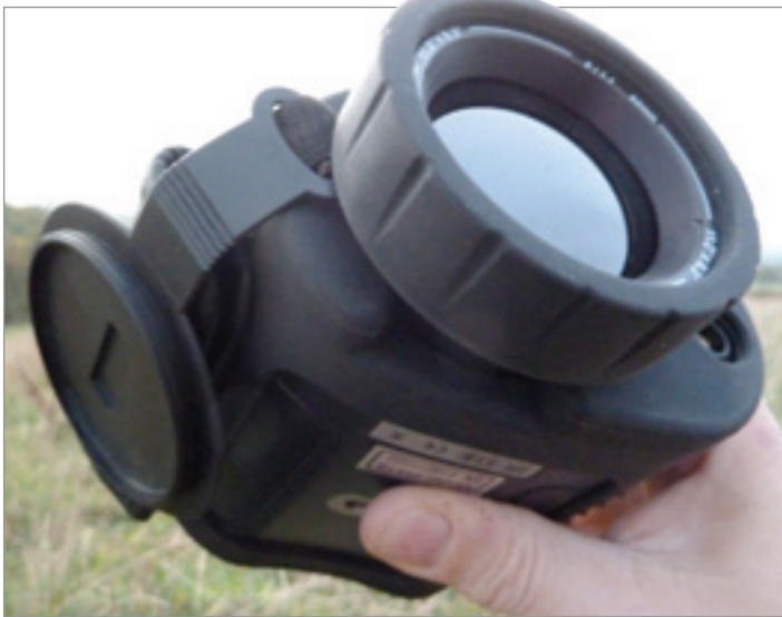
The IR518 is also available with a 25mm lens but this top-of-the-line "C" model has a more powerful, 50mm lens, focusable from a few feet to infinity
