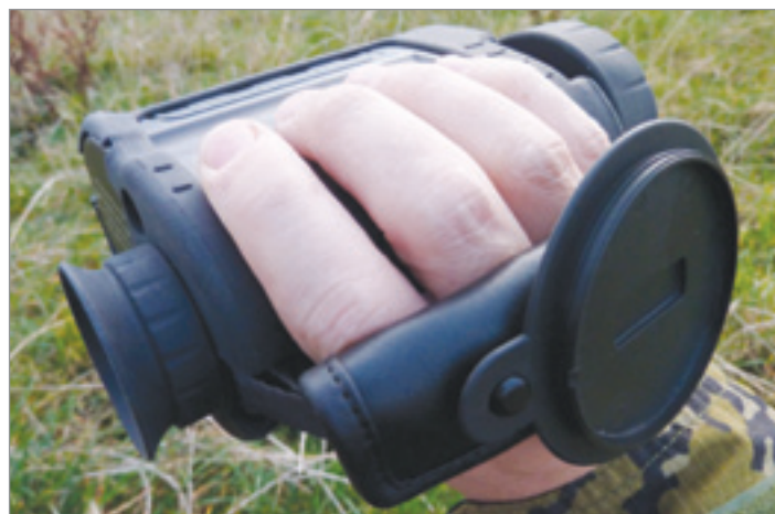
An adjustable hand strap frees your fingers to operate the buttons and incorporates a stud for securing the lens cover when open
