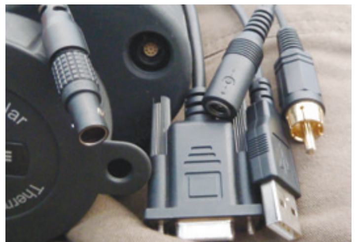
A single port in the front of the housing takes a cable that both supplies power and lets you connect to an external monitor via a choice of three formats
