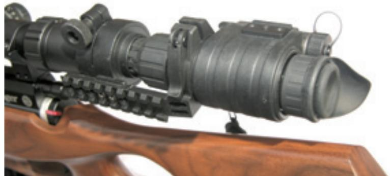
**The Challenger 1 X 20 Monocular now simply pushes into back of DSA until it abuts up flush to opposing side - note Weaver Rail for fitting additional kit, higher intensity IR's, lasers etc...**
