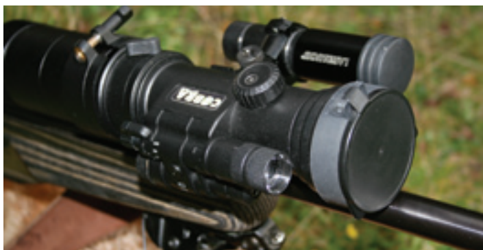
Built in IR illuminator on the right side with the focus wheel visible on top of the body at the front. An optional LaserLuch illuminator is fitted to the left on the Weaver rail
