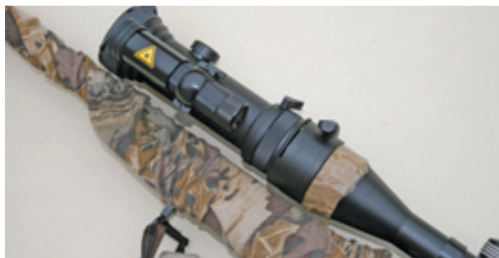
On the Kahles scope I had to pad the objective lens to stop it moving backward
