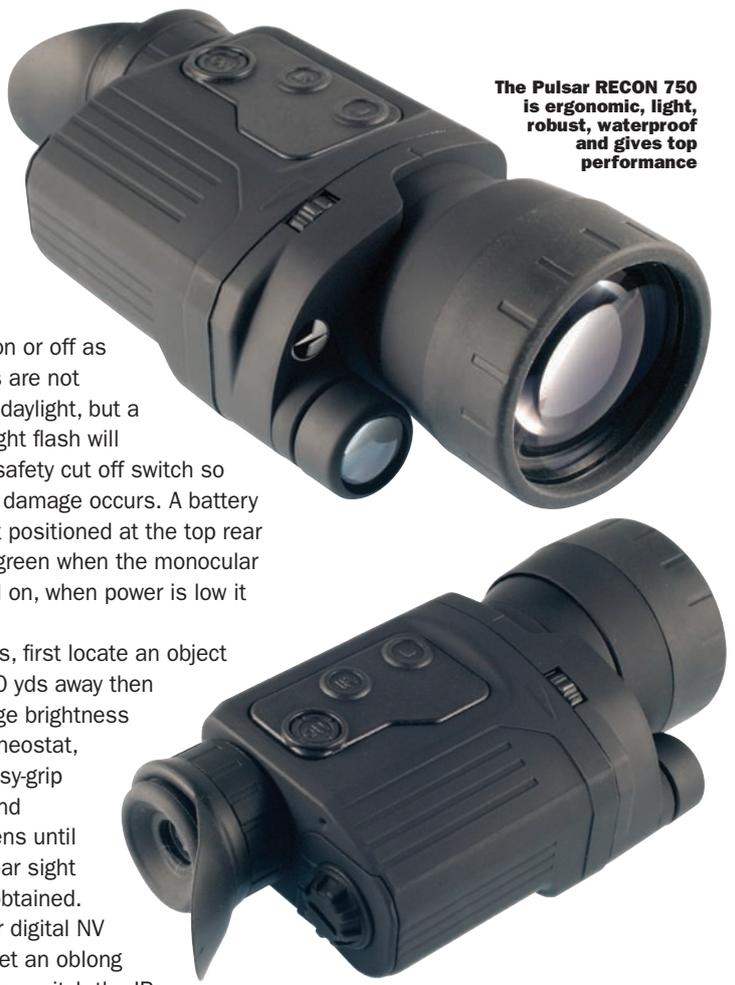
Pressure pad control switches and rheostat are much simpler to use than the 'recordable' relatives, and exactly where they need to be as you hold and use it
